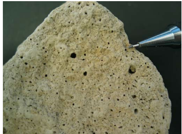
Figure 10. Sample of clay recovered from 25 feet below ground surface after 30 days heating by ERH. Steam bubble formation and escape created microfractures and vuggy porosity. It was noted that the vacuum pressure on the subsurface decreased and the flow rate increased as heating of the clays progressed, with concurrent release of steam and vaporized contaminants (McGee et al., 2006).
