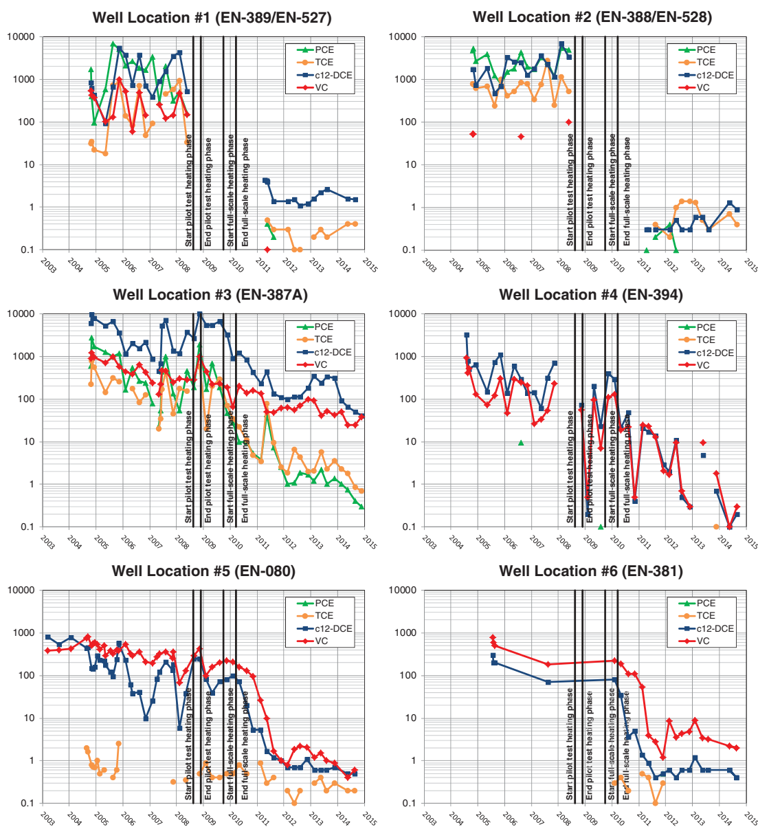
Figure 6. PCE-series groundwater concentrations in source area and plume area before and after thermal treatment. Monitoring well locations are shown in Figure 2.
