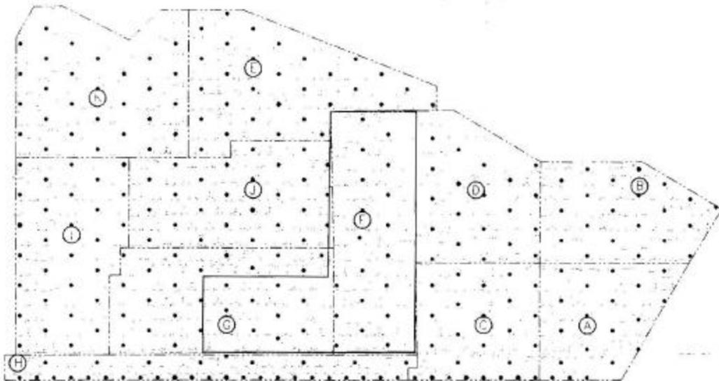
**FIGURE 1. Locations of heater (open circle) and vacuum/heater (closed circle) wells on 7-foot triangular spacing. Heavy line shows L-shaped office (left) and warehouse (right). Light lines delineate property boundaries. Dashed lines indicate separate process control areas A-I for ISTD well fields.**
