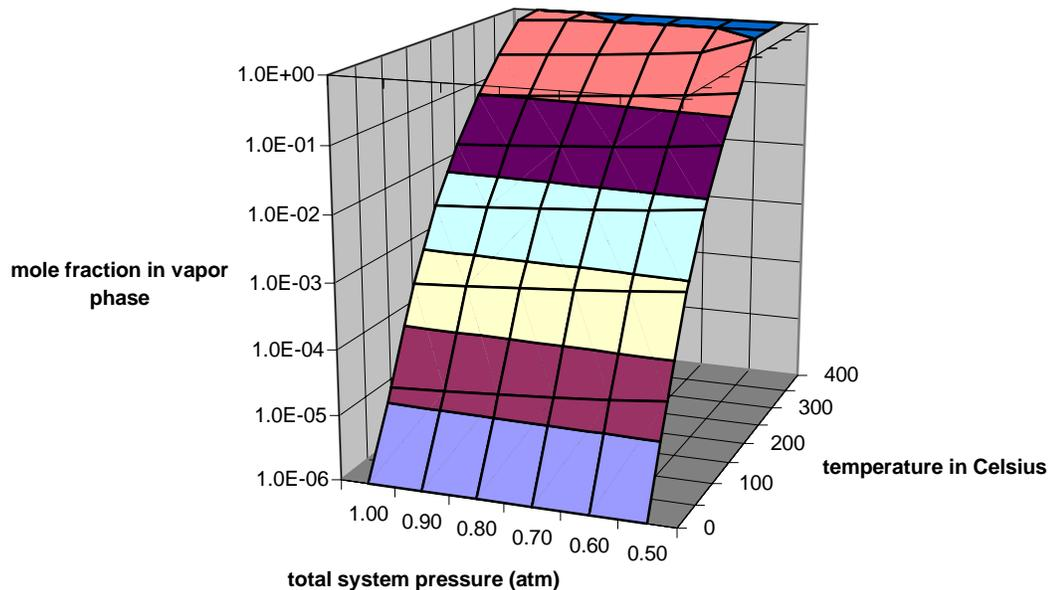
Finally, at 250°C, the vapor stream in equilibrium with liquid mercury contains 450 grams per cubic meter, or almost 13 grams of mercury per cubic foot, and is over 40% by weight mercury. It is achievement of temperatures above this threshold that allows ISTD to comprehensively remove the mercury from subsurface remediation sites.
