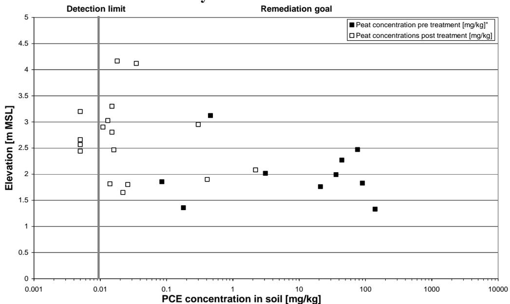
**Figure 5. Pre and Post Treatment Soil PCE Concentrations with Depth Relative to the Mean Sea Level for Peat Samples. Note that the X-axis is Logarithmic. Non-Detect Samples are Shown in the Graph with a Value Corresponding to Half the Analytical Detection Limit.**
