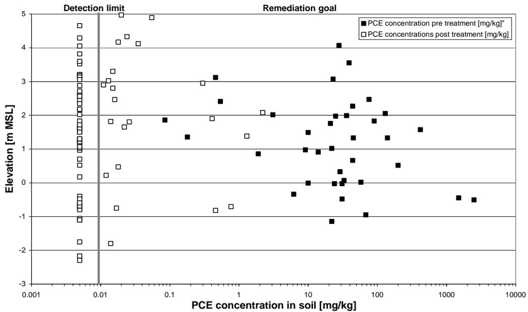
**Figure 4. Pre and Post Treatment Soil PCE Concentrations with Depth Relative to the Mean Sea Level (MSL). Note that the X-axis is Logarithmic. Non-Detect Samples are Shown in the Graph with a Value Corresponding to Half the Analytical Detection Limit.**
