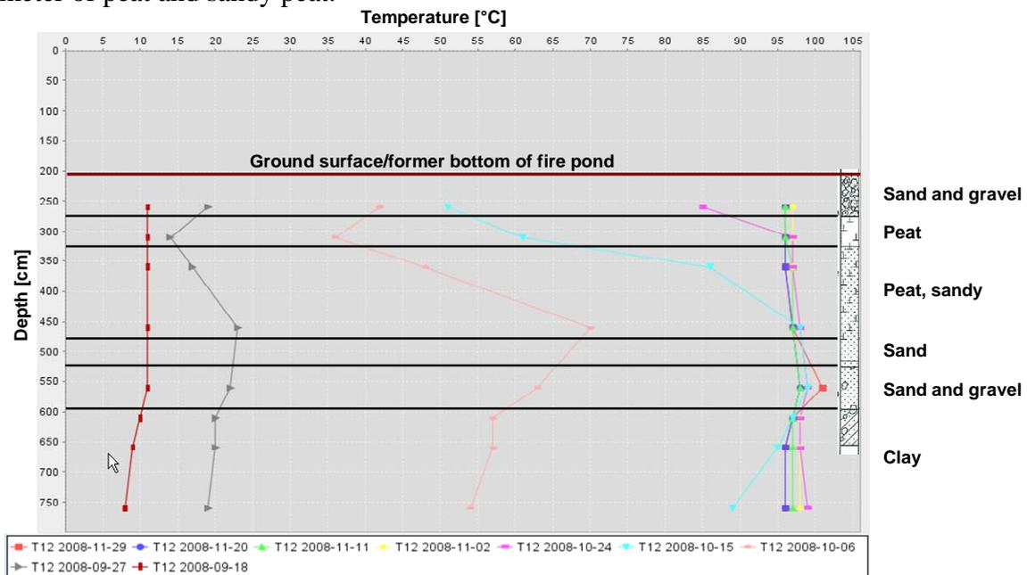
**Figure 3. Temperature Profile at T12 Located in Peat Area.**
