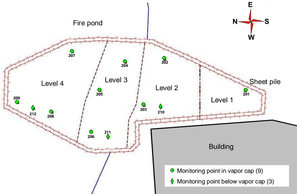
**Figure 7. Location of 12 Leveling Points Used to Measure Subsidence During Treatment.**
