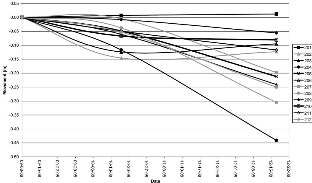
**Figure 8. Surveyed levels for the 12 locations during ISTD treatment.**
