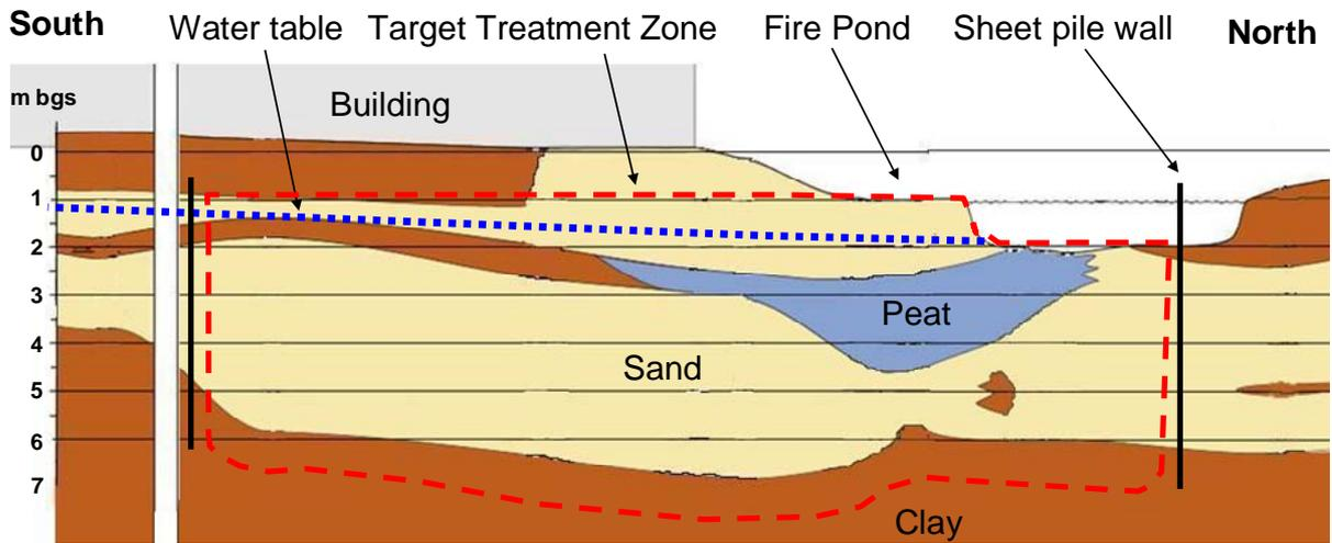
**Figure 1. Conceptual Treatment Area Cross-Section.**
