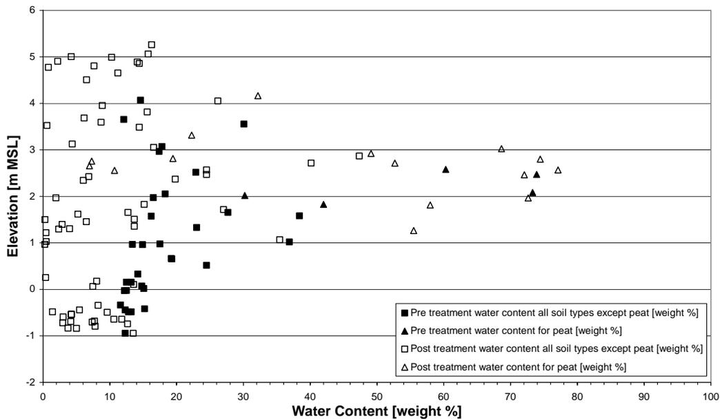
**Figure 6. Soil Water Content Prior to and After Treatment by Depth Relative to the Mean Sea Level.**
