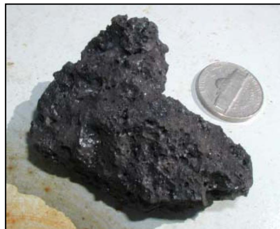
Close-Up of Stabilized Coal Tar from just above the Bottom of the Gasholder
